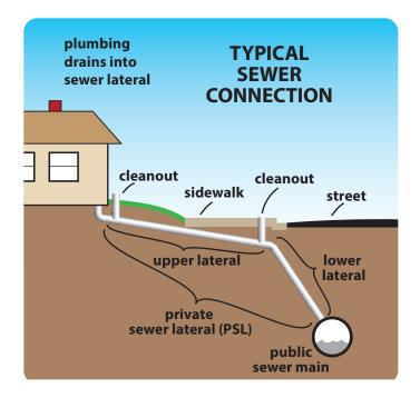
A private sewer lateral (PSL) is the pipe that carries waste from the plumbing in a home or business to the sanitary sewer main, usually located in the street. It consists of two sections: an upper lateral, which connects the building cleanout to the curbside cleanout, and a lower lateral, which connects the curbside cleanout to the sewer main. Property owners are responsible for maintaining the entire PSL, except in Alameda and Albany where that responsibility is for the upper lateral only.
