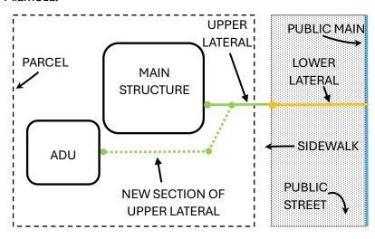
If your property does have a valid, unexpired Compliance Certificate, the permitting authority may require you to test any new PSLs or sections of PSLs installed. For example, if a new section of upper lateral was installed from the lateral serving the main structure to the new ADU, this section may need to have pressure testing witnessed by an EBMUD inspector. After the new PSL section(s) pass
